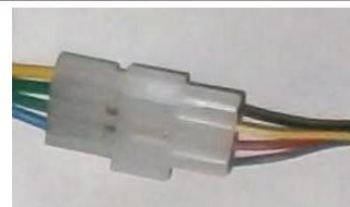
Power on machine. Pull apart encoder connector at motor.
