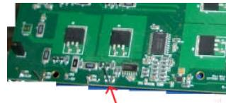
Move the black lead of meter to gnd test point on mmc **GND TEST POINT** or tmc
