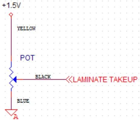
To determine if the problem is the control pot or the webamp board you can use a DVM set to DC volts with black wire connected to GND on connector (blue wire on photo) measure the voltage at pins 2, 3, 4 or 5 on J10. As you turn the associated pot on the front panel the voltage on the control pin should change between 0V and about 1.5V. If the voltage changes the problem is on the board. If the voltage does not change the problem is in the pot.
