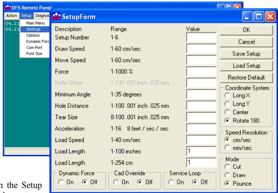
To save a custom set-up simply fill in the desired value(s) in the appropriate window, including the Setup Number, click on the **Save Setup** button.
