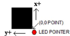
The i-TECH uses a special HPGL command, FO, to start the registration mark sensing function. It automatically re-registers the coordinate each time the FO HPGL command is received. As part of the setup a “x move between jobs” is input via the printer driver options which moves the sensor to the approximate position of the next copy’s or next frame’s registration mark. The i-TECH expects the target for the next frame to be within ½ the scan distance of the end of the frame.
