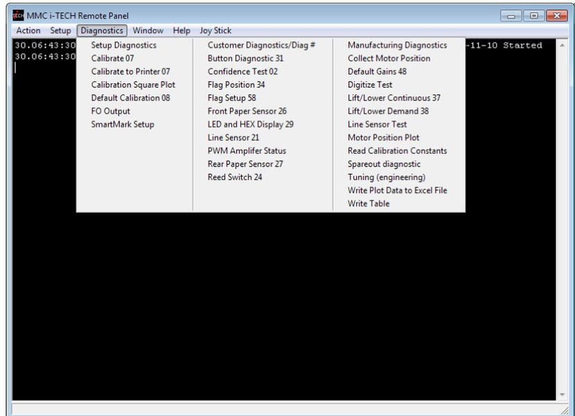
**IMPORTANT!! DO NOT run Manufacturing Diagnostics unless specifically instructed by direct contact with Allen Datagraph Technical support. Damage to the system is possible if not run correctly.**
