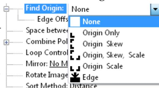
**Origin Scale** does alignment at the origin, rotation and x-axis only scaling at the scale point. It assumes that the scaling in the y-axis is correct. If the printer you are using has a x axis scaling error you can normally correct this either in the printer or you can use calibrate to printer to get the cutter to cut the same size as the printer.
