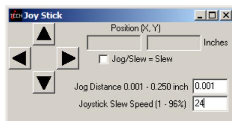
so that Jog/Slew = Slew, the joystick speed will be the speed set in the Joystick Speed Window. Left Click and hold the arrow button to move the material or carriage. With the Jog/Slew box checked so that Jog/Slew = Jog, the arrow buttons will jog the cutter that fixed distance each time the button is clicked.
