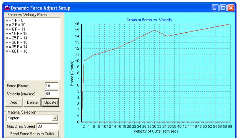
and Velocity Window, type in the desired force vs. velocity that you have established for the material. The recommended method for establishing the various force vs. velocity numbers is to run the test cut at various velocities and record the results for entry here.
